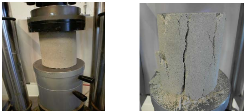
Figure 4.1 Monotonic compressive testing and specimen after failure
