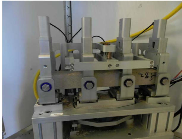
Figure 4.23 Four-point bending test setup
