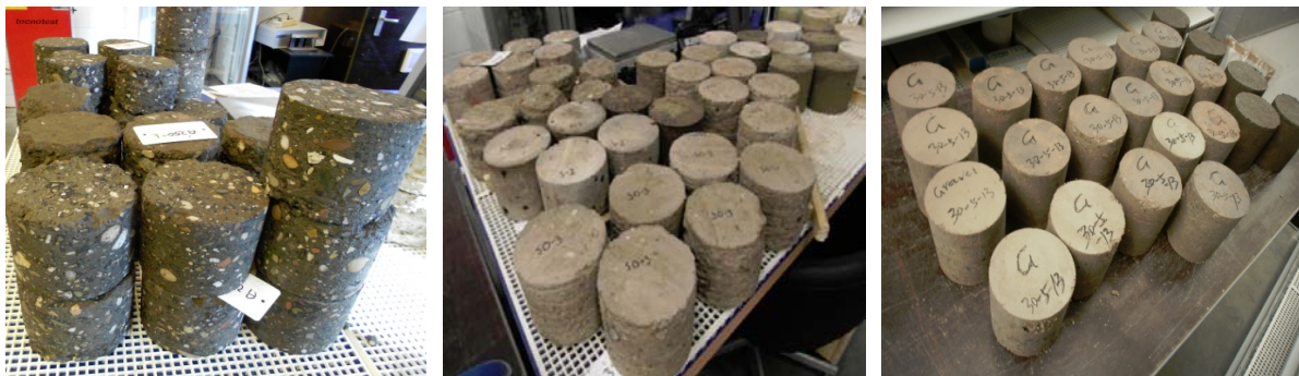
Figure 7.18 Field cores (left and center) and laboratory-prepared specimens (right)
