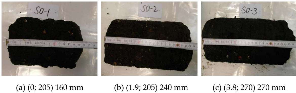
Figure 7.30 Field cores of stabilized in-situ sand at 28 days ( M=121^{\circ}\text{C}\cdot\text{day} )
