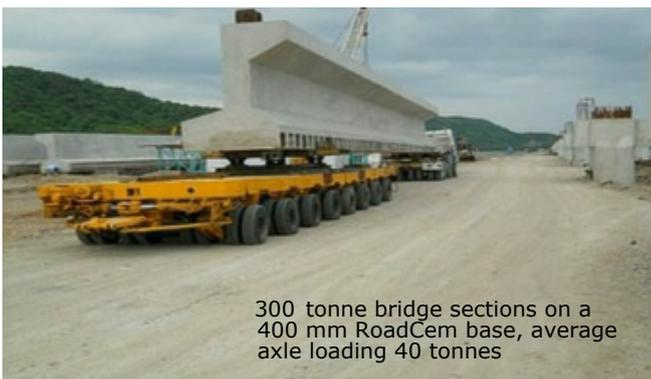
300 tonne bridge sections on a 400 mm RoadCem base, average axle loading 40 tonnes
